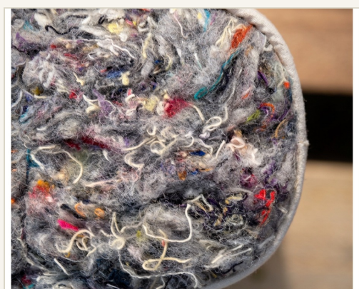
Cross-section: the core is built from recycled textile fibre.
